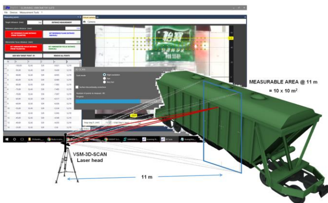
VSM-3D-SCAN optical heads with mechanical mount (left). PC software and measurable area (right)
