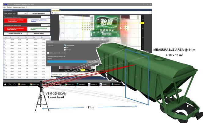
VSM-4000LL-3D-SCAN-TRACK-EXT optical heads (left). PC software and measurable area (right)
